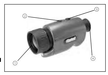
Direct the device at an object at a distance approximately 100 yards and rotate the eyepiece (4) to give the best quality image. After the adjusting, do not rotate the eyepiece any longer irrespective of the distance and other conditions.
